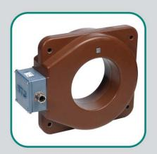
Window type and slip on type current transformers are applicable when the path for current is the existing cable or busbar which is not possible to be cut for the insertion of a normal CT.
